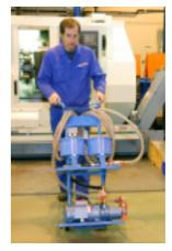
Mobile low pressure filter system used to remove particles and water contamination from hydraulic systems with the ability to move from one machine to another. Can also transfer, without filtration, of large & small quantities of used oil from hydraulic system reservoirs to storage for disposal.
