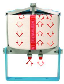
The high tech cartridge gives continuous all round protection against water and ultra-fine debris with contaminated oil entering the filtakleen unit at the base flowing up the centre tube through the 1 micron filter before flowing back to the hydraulic circuit. Flow rates through filter 4.1 I/min to 6.1 I/min depending on unit fitted.
