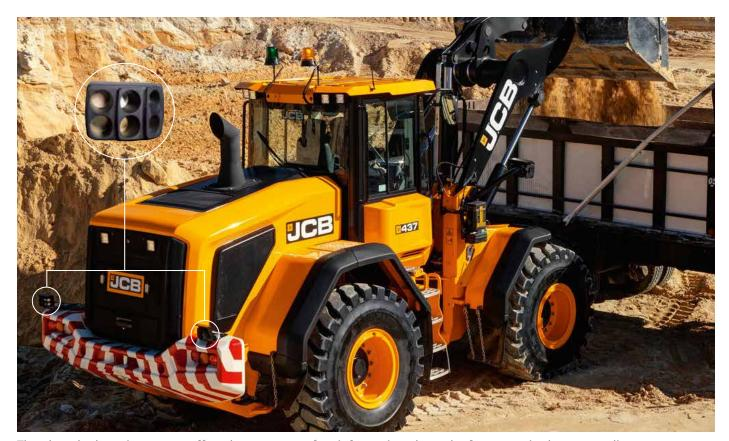
The obstacle detection system offers the operator safety information about the free space in the surroundings of the machine.
