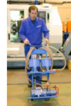
Mobile low pressure filter system used to remove particles and water contamination from hydraulic systems with the ability to move from one machine to another. Can also transfer, without filtration, of large & small quantities of used oil from hydraulic system reservoirs to storage for disposal.
