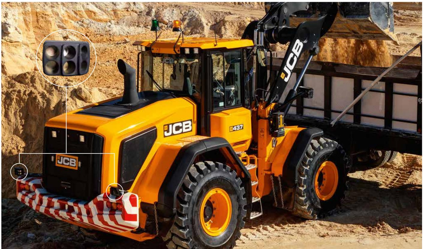
The obstacle detection system offers the operator safety information about the free space in the surroundings of the machine.
